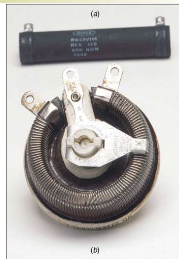
Fig. 2-3: Large wire-wound resistors with 50-W power ratings. (a) Fixed R , length of 5 in. (b) Variable R , diameter of 3 in.
