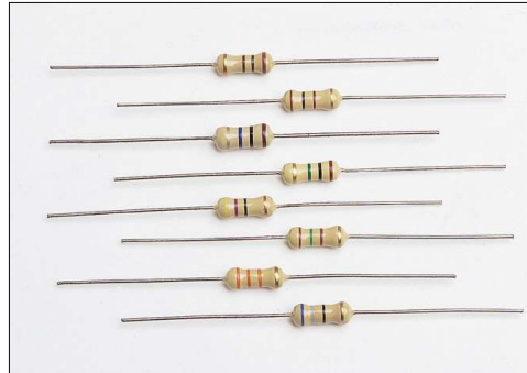
Fig. 2-2: Carbon resistors with the same physical size but different resistance values. The physical size indicates a power rating of \frac{1}{2} W.
